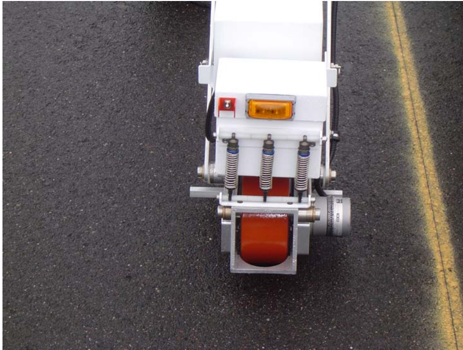
ICC Surpro – wide tire (close-up view).
