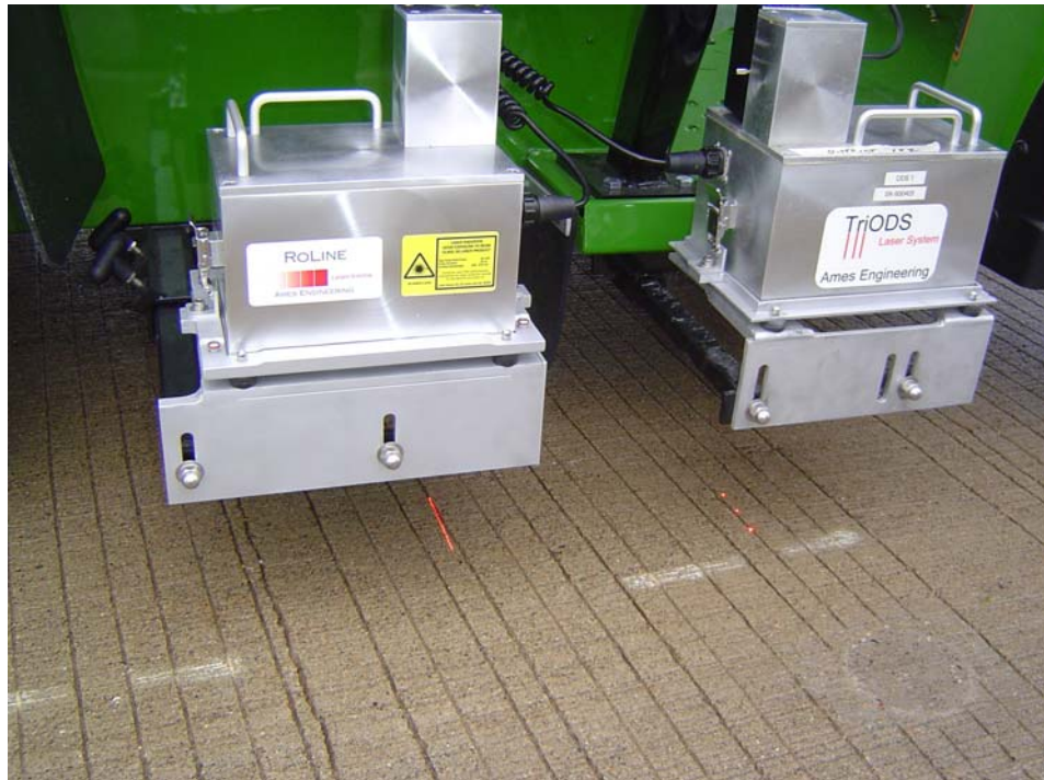
RoLine and TriOD sensors mounted on the Ames lightweight profiler.
