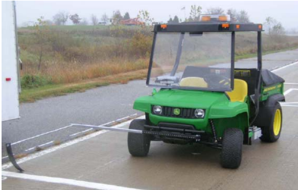
Ames lightweight profiler with guidance system.
