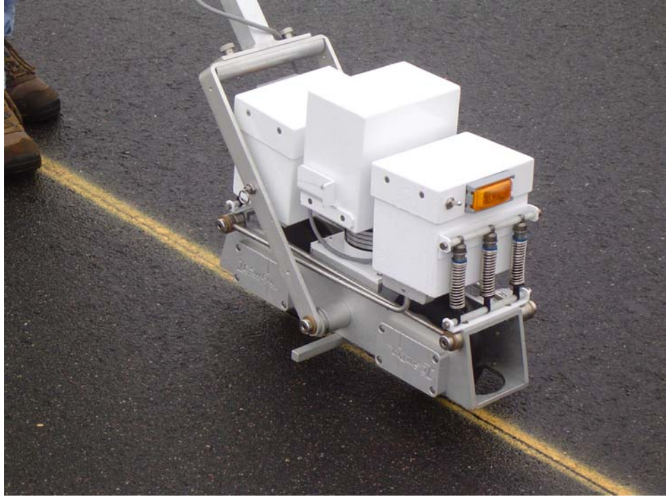
ICC Surpro – normal tire (close-up view).
